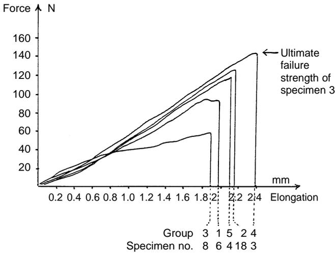
**Fig. 3** Force/elongation diagram of one example specimen for each group
